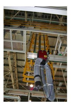
Full Automatic Vertical Shifter ensure the transfer of the hose trolleys between two return rails located at different levels.
