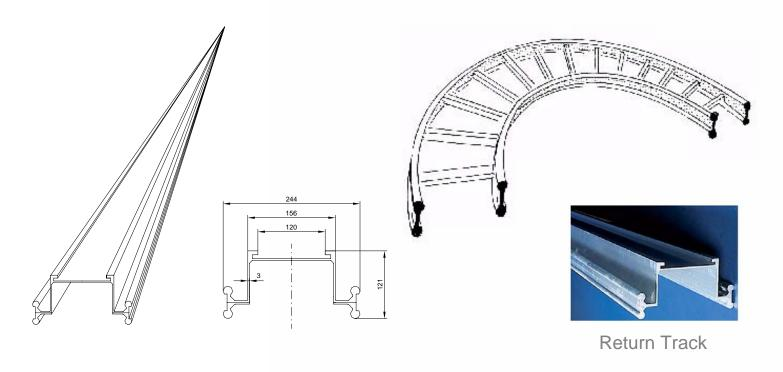
Return Rail made of extruded Aluminium. Any length available. Weight: 7,5 kg/m Return Rail - Bend Available radius: 1.200 / 1.500mm from 15° to 180°
