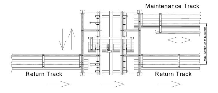
Full Automatic Horizontal Shifter ensure the transfer of the hose trolleys between two or more suction ducts and/or return rails installed parallel to each other. Maximum safety due to two-ways locks, limit switches and overload protection.
